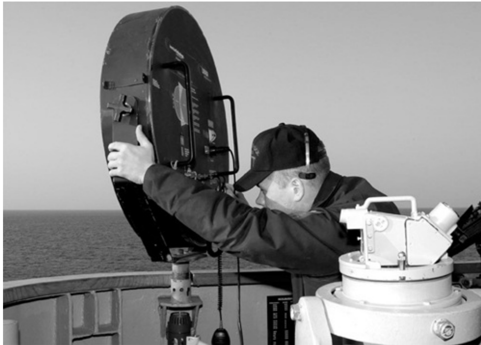
A Long Range Acoustic Device used onboard the USS Blue Ridge during a small boat attack drill, 2006. U.S. Navy image.
