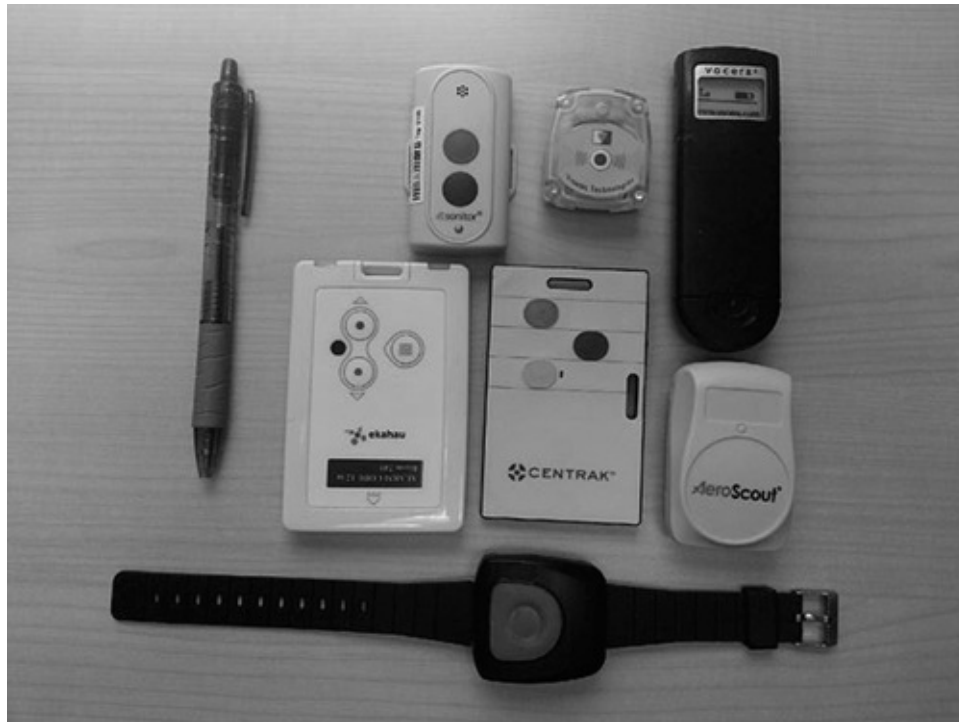
A collection of commercially used RFID tags. Wikipedia image made available under the GNU Free Documentation license.
